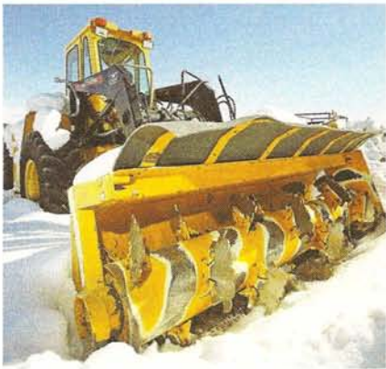
A Brown Bear composter is used to aerate and windrow biosolids before application on tribal agricultural lands.
